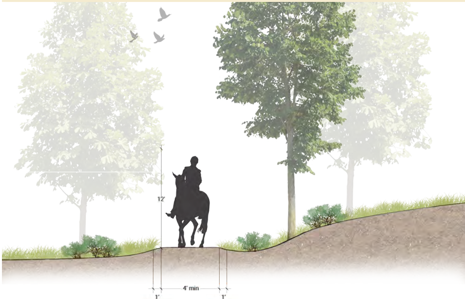
FIGURE 5.11 - UNPAVED/EQUESTRIAN TRAILS - TYPICAL SECTION
