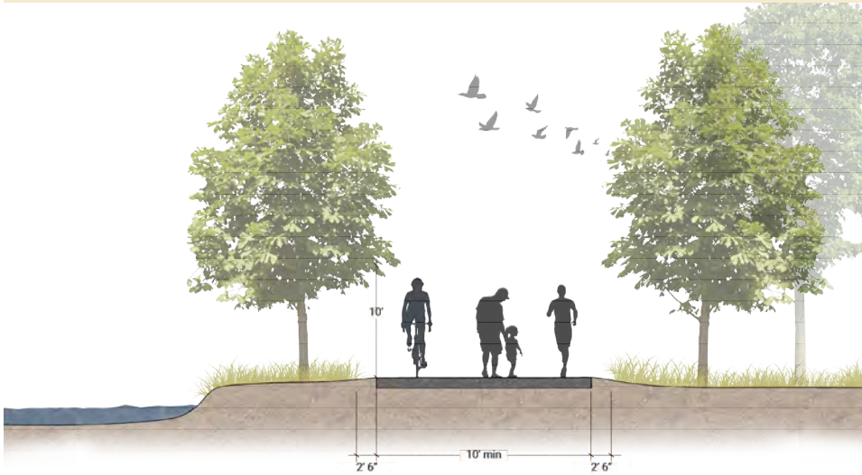
FIGURE 5.10 - REGIONAL AND LOCAL TRAILS - TYPICAL SECTION
