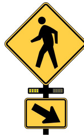
FIGURE 45: RRFB Design (Source: MUTCD Figure 4L-1)
